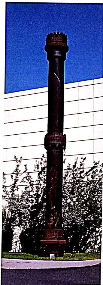
Historical first pressure steel reactor used for ammonia production by Haber in 1921
